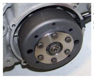
In that position, fasten the rotor carefully with the original nut.
