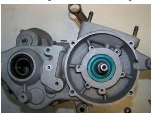
Unscrew the old stator and take it off the engine. Pull the rotor off, you will need a puller for this.
