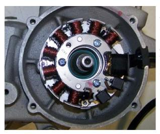
Put the stator coil back onto the plate, take care not the damage the wires. the stator has to snap in rather sharply. If it sets soft, you have probably jammed a wire underneath!
