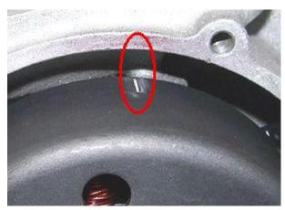
Place the rotor loosely onto the crank and check that it may move freely above the statorbase.
