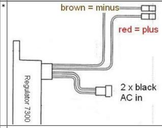
The new regulator/rectifier has 4 wires
